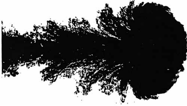
FIGURE 15. Flow visualization of a turbulent vortex ring. (A. Glezer & D. Coles 1987, private communication.)
